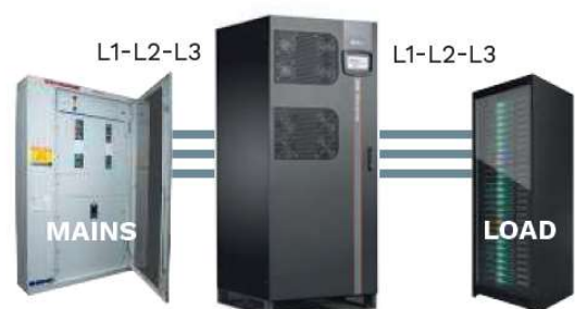
3-wire (L1-L2-L3) installation
