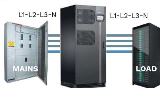
4-wire (L1-L2-L3-N) installation
